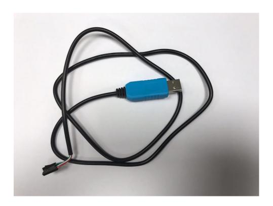
Settings at this "serial-debug-port" are: 115.2 KBaud, 8, N, 1 – no flow control (that is what worked for me)
